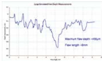
Figure 8: Profile measurements of simulated flaw (right).
