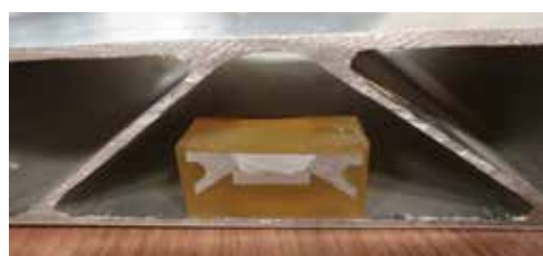
Section through a floor extrusion plus an early prototype weld repair macro from procedure qualification.
