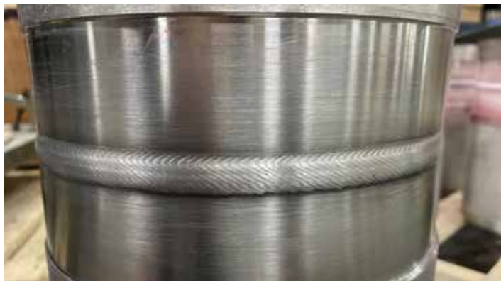
Figure 2: Completed weld profile.
