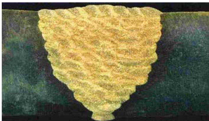
Figure 4: A WPQR microsection through a GTAW welded joint from a 609.6 mm (24" NB) x 62 mm thick Hot Isostatically Pressed ZERON 100 SDSS injection manifold [7]. Courtesy, Rolled Alloys.
