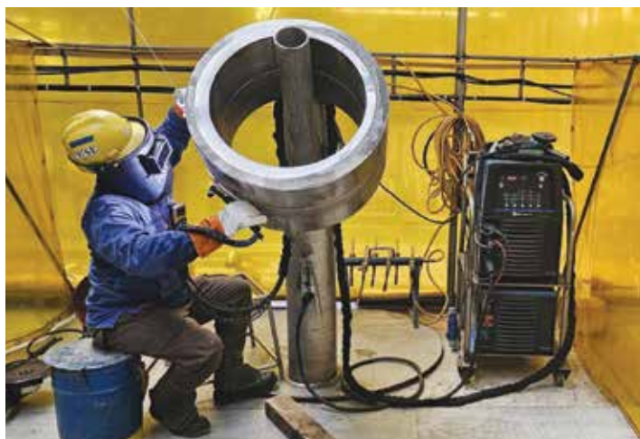
Figure 5: Welding procedure qualification test piece in a thick wall SDSS pipe. Courtesy, Equinor [9].
