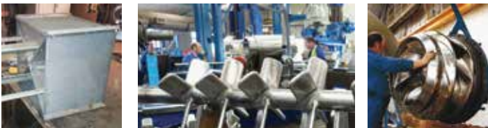
Figure 3: Left: Vortex breaker. Middle: Phosphoric acid agitator/mixer. Right : FGD pump impeller. Courtesy, Rolled Alloys.
