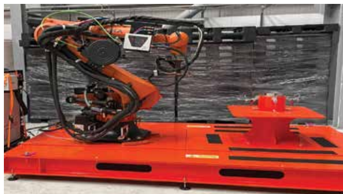
Figure 5: TANICS™ welding robot on transportation skid.
