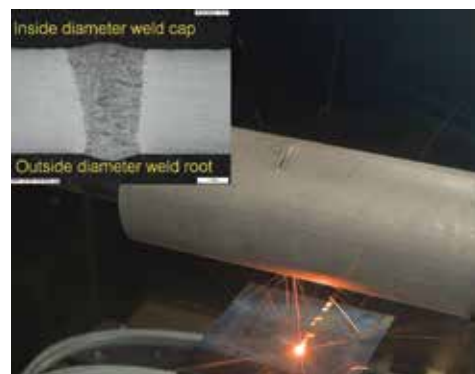
Figure 3: Internal welding set-up showing beam path within the EBOBend device.
