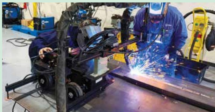
Figure 4: Hercules GMAW process running on a Gulco SAM Carriage.
