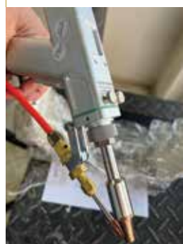
Figure 1: Typical handheld laser torch equipped with wire feeding system.
