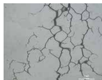
Figure 5: Micro-section through crack tip at higher magnification, detailing intergranular cracking.
