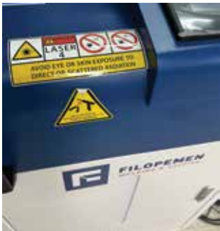
Figure 2: Handheld 2 kW laser welding equipment - safety signs.
