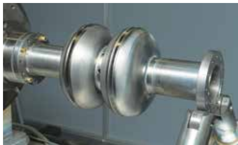
Figure 5: Electron beam welded twin-cell demonstration SRF cavity.
