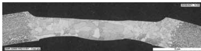
Figure 10: Equator weld in SRF cavity.
