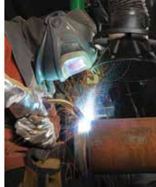
Figure 2: MAG welding with adjustable local exhaust ventilation. Courtesy TWI Ltd.
