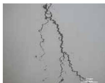
Figure 4: Micro-section through the crack tip, showing the branched crack.
