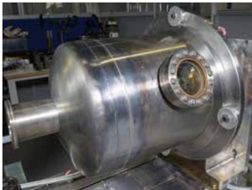
Figure 14: Stainless steel vacuum vessel used for internal welding trials.
