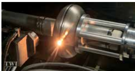
Figure 6: Repair simulation set-up for a single SRF cavity.
