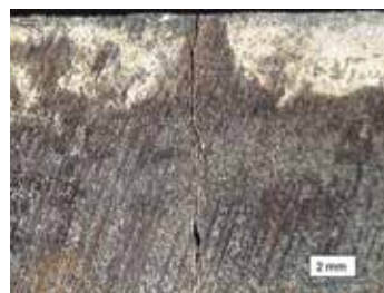
Figure 2: Macro image showing longitudinal crack at internal surface of plate.
