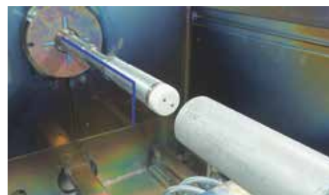
Figure 3: Internal welding set-up showing beam path within the EBOBend device.
