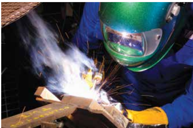
Figure 1: Fume arising from MMA welding. Courtesy: TWI Ltd.
