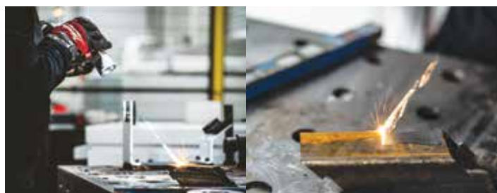
Figure 3: Laser removal of cutting scale from a weld bevel. Copyright Fanuc & Falcon.
