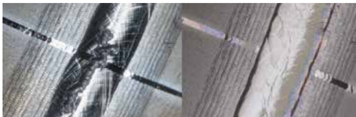
Figure 9: Internal repair of niobium cavity: before and after processing.
